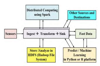
FIGURE 2. IoT architecture. Data collected by sensors can be sent to different systems which use various software platforms to carry out intended tasks [38].
