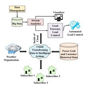
FIGURE 5. System architecture for load shedding and smart load controlling algorithm [58]. All the components of the system are connected to the cloud which makes decisions based on the system inputs, and sends out commands for execution. The directions of the arrows indicate the flow of data.
